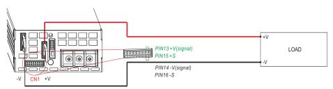
2. Output Voltage Programming (or, PV / remote voltage programming / remote adjust / margin programming / dynamic voltage trim)
